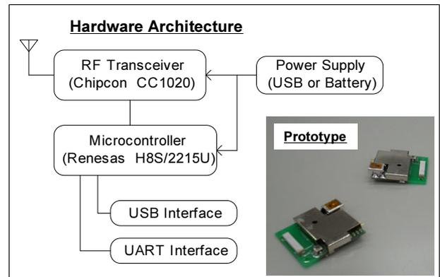
Figure 1: Overview of the U<sup>1</sup>-Chip
