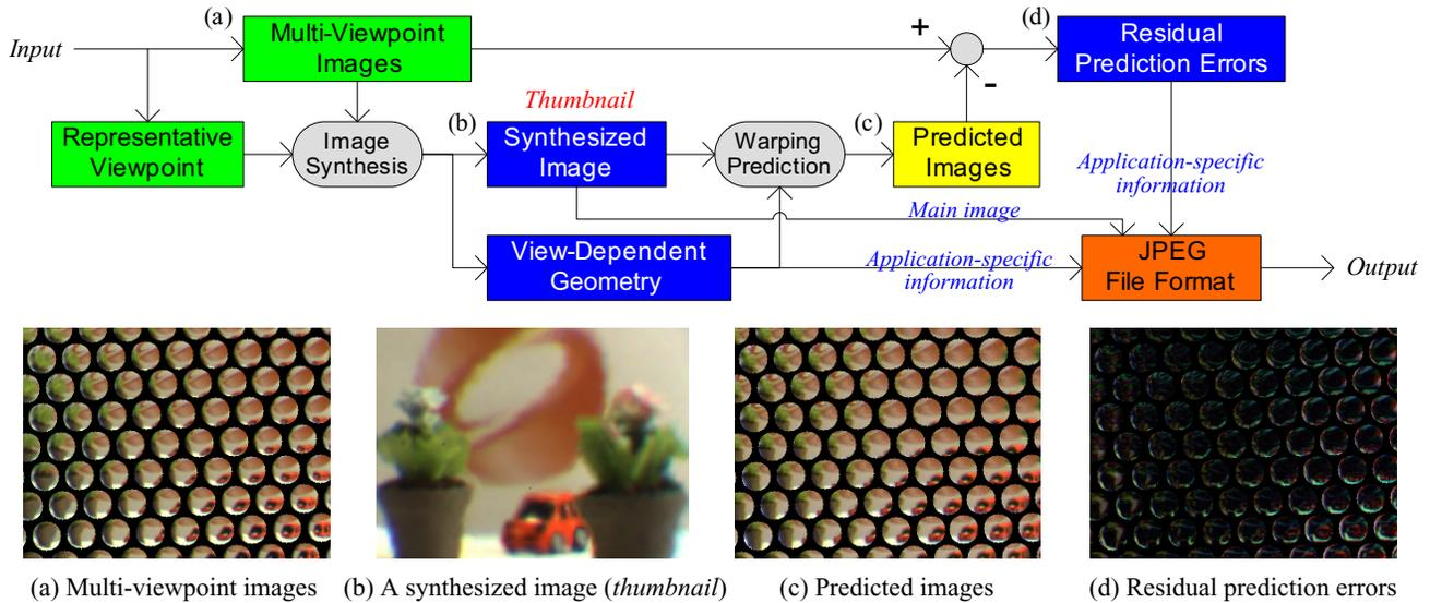
Figure 1: A block diagram of the proposed coder (top) and example images using an integral photography (bottom).
